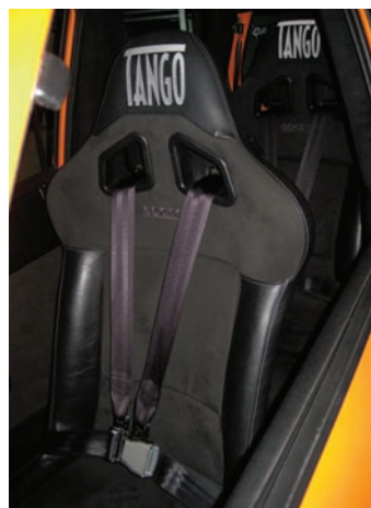
Four-point pilot’s harnesses on both front and rear seats with inertia reels are similar to those used in racing, but easy to get into. (below)
