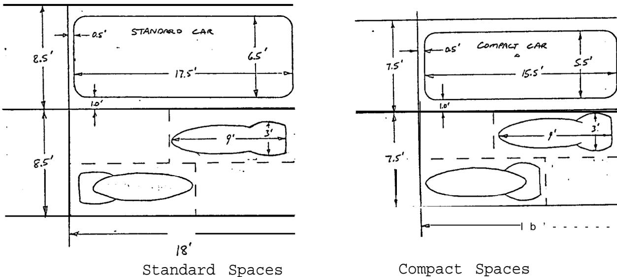
Figure 1. The Lean Machine in Existing Parking Spaces.
