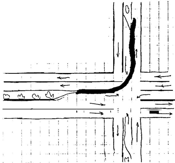
**Figure 4.** Intersection of an East-West Four Lane Arterial Highway and a North-South Local Street. Left turn lanes are provided for conventional vehicles. Additional capacity for eastbound to northbound turns is provided by a flyover for Lean Machines.
